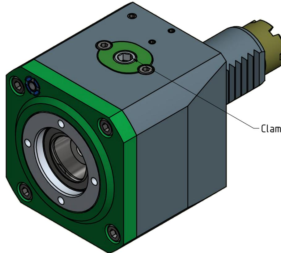
Clamping torque 35 Nm
