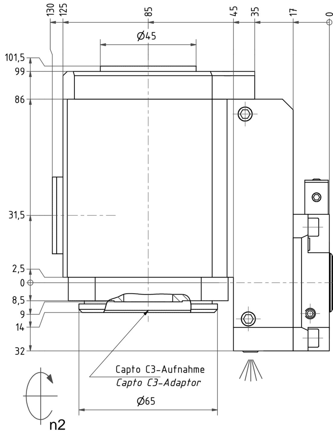
Clamping torque 35 Nm
