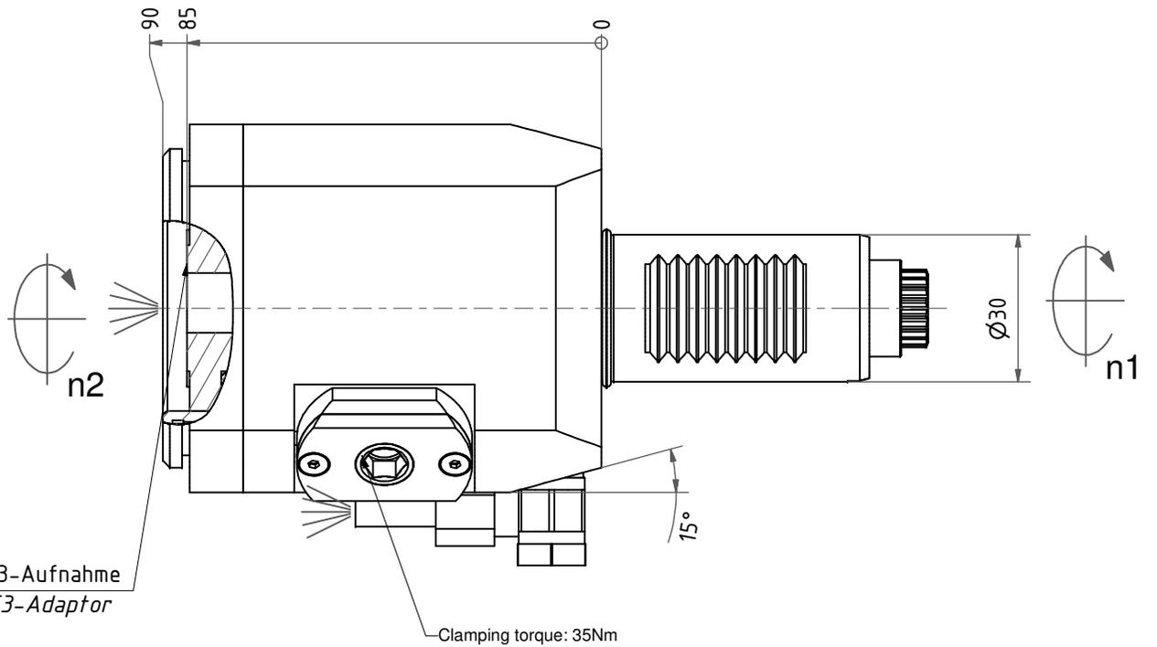
Clamping torque: 35Nm
