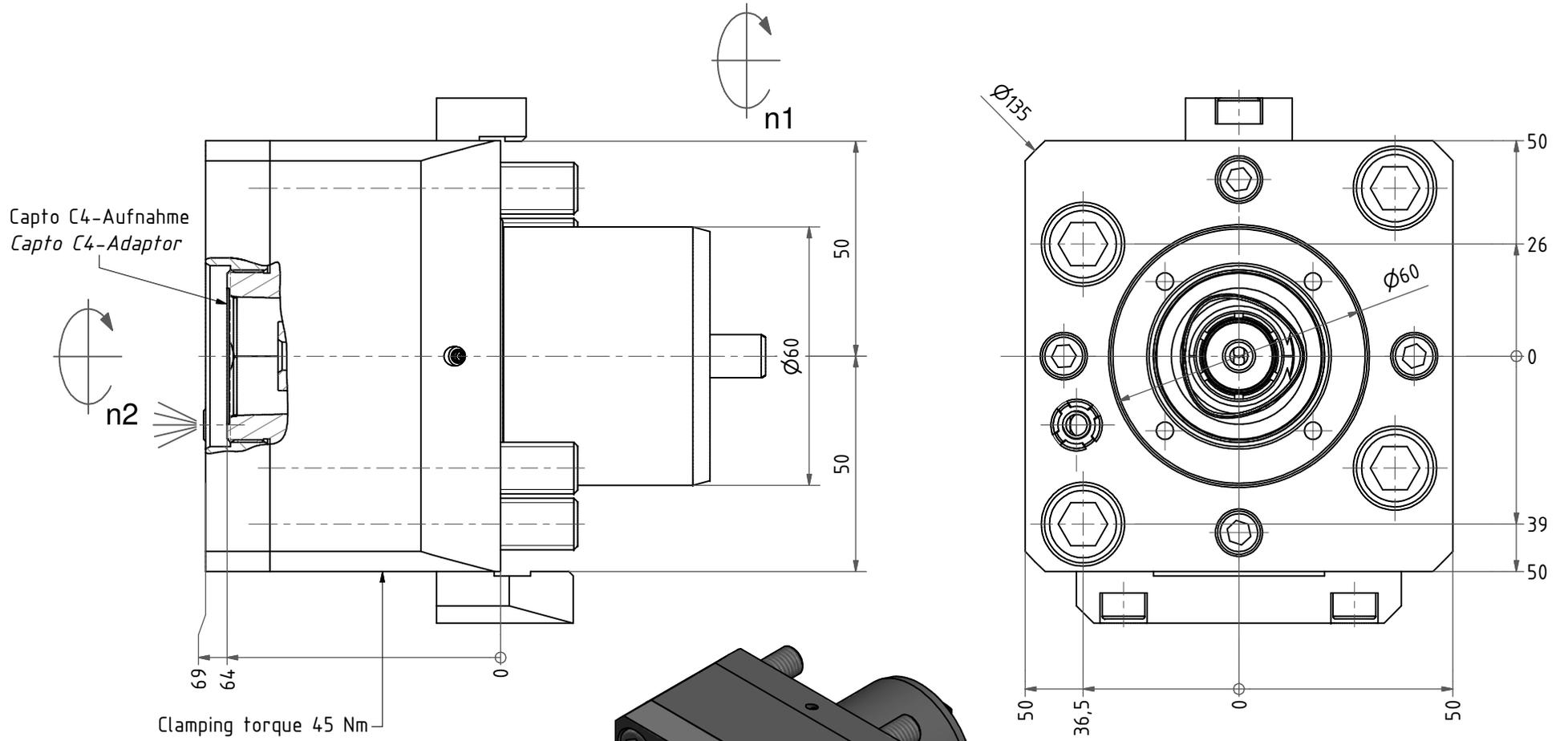
Clamping torque 45 Nm
