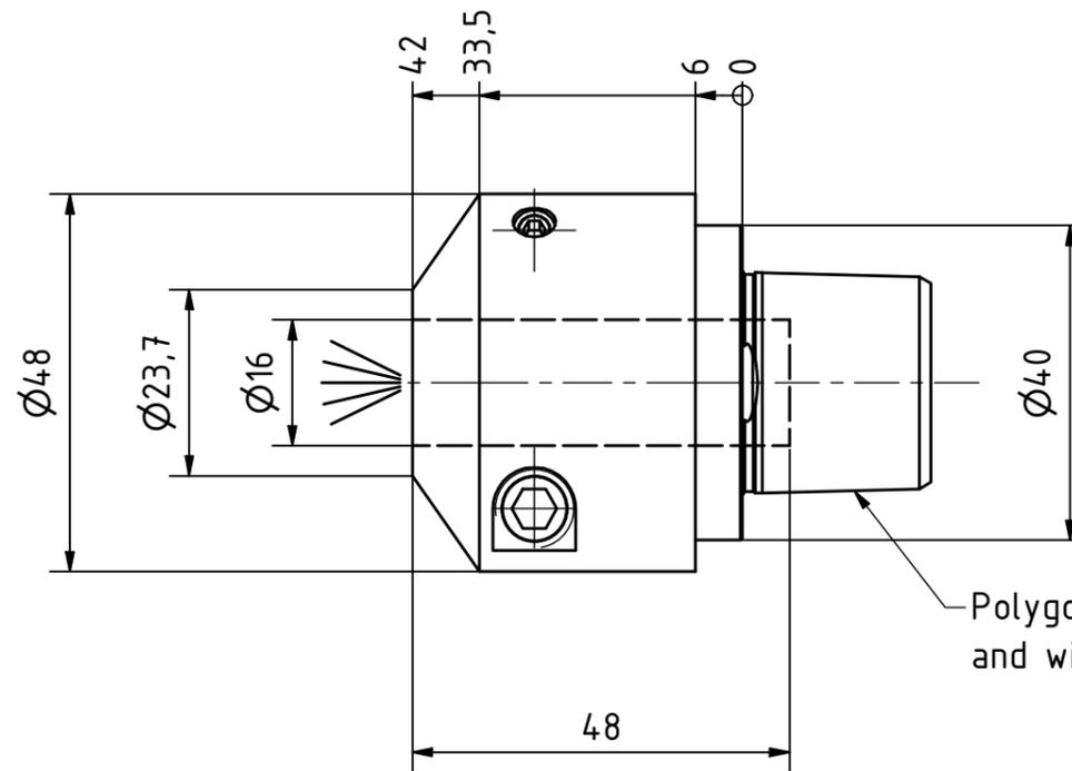
Polygon ISO 26623 PSC 40 without thread and without gripper
